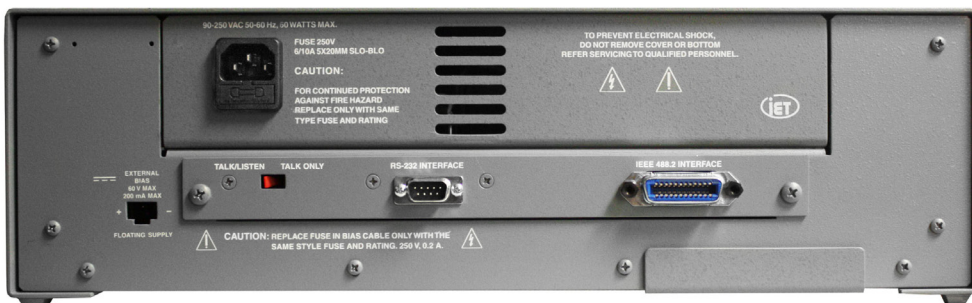
Rear view of 1689 RLC DigiBridge with optional IEEE-488 interface
