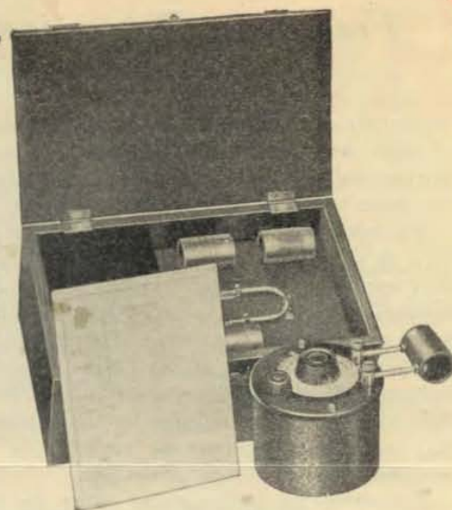
FIGURE 2. THE TYPE 558-P METER CONTAINS NO RESONANCE INDICATOR
