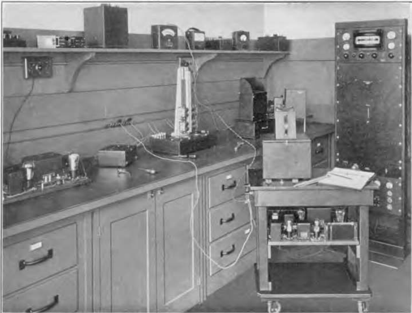
FIGURE 3. A laboratory set-up. A study is being made of the performance of a number of tube-driven tuning forks. The relay-rack panel includes a constant-temperature container for housing a precision fork. A stroboscope accurately comparing two frequencies is shown in the foreground
