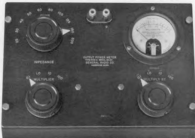
FIGURE 1. Panel view of a TYPE 583-A Output Power Meter, showing the available impedance settings and the meter scale
