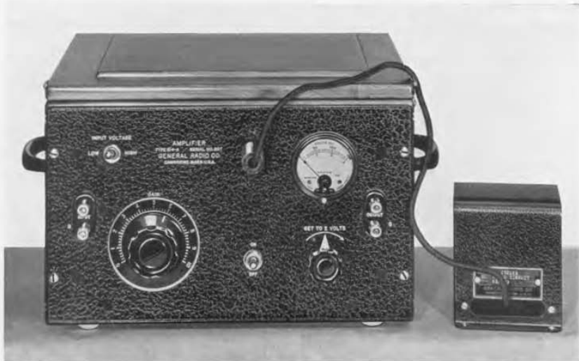
FIGURE 1. Showing how the tuned circuit is plugged into a jack on the amplifier panel
