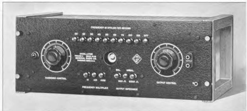
FIGURE 1. Panel view of the TYPE 608-A Oscillator. Both frequency and output impedance are selected by means of push-button switches.
