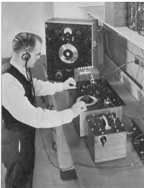
FIGURE 2. Calibrating a TYPE 722 Precision Condenser in the Standardizing Laboratory.
