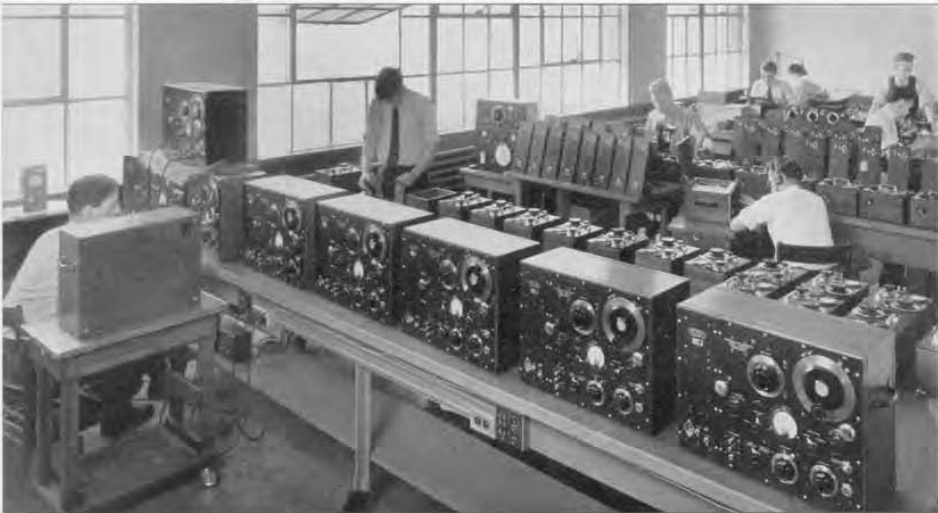
FIGURE 1. View of a portion of the Standardizing Laboratory, showing a group of TYPE 605 Standard-Signal Generators undergoing test and calibration.
