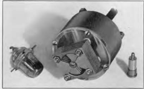
FIGURE 11. 900–3000 Mc butterfly circuit. Acorn tube and 1N22 detector are shown for size.
