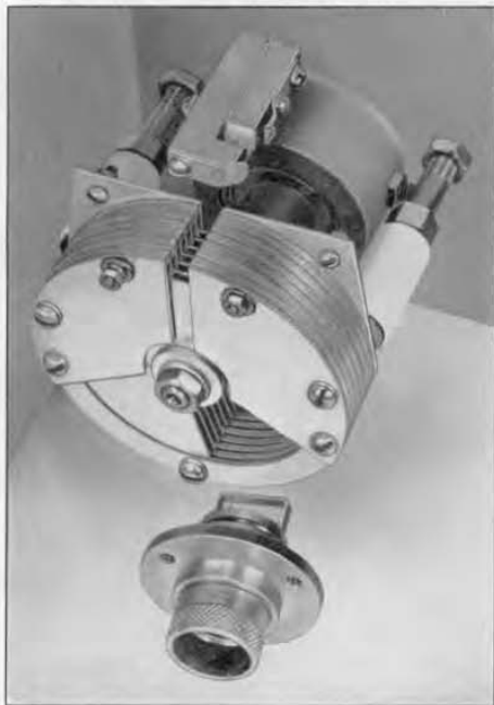
FIGURE 7. 100-500 Mc Oscillator. Inductive coupling to the load is varied by rotation of the coupling loop in lower part of the picture.
