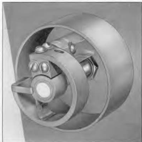
FIGURE 3. 400-1600 Mc. Wavemeter. End of stator band connected to rotor.
