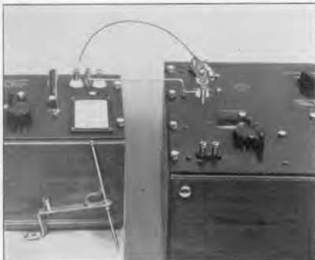
Figure 2. This fine wire connector, by means of which Curve A of Figure 5 was obtained, is used in calibrating all precision capacitors in our laboratories. An older type of connector is shown leaning against the capacitor cabinet and produces a much greater error as shown in Curve B of Figure 5.
