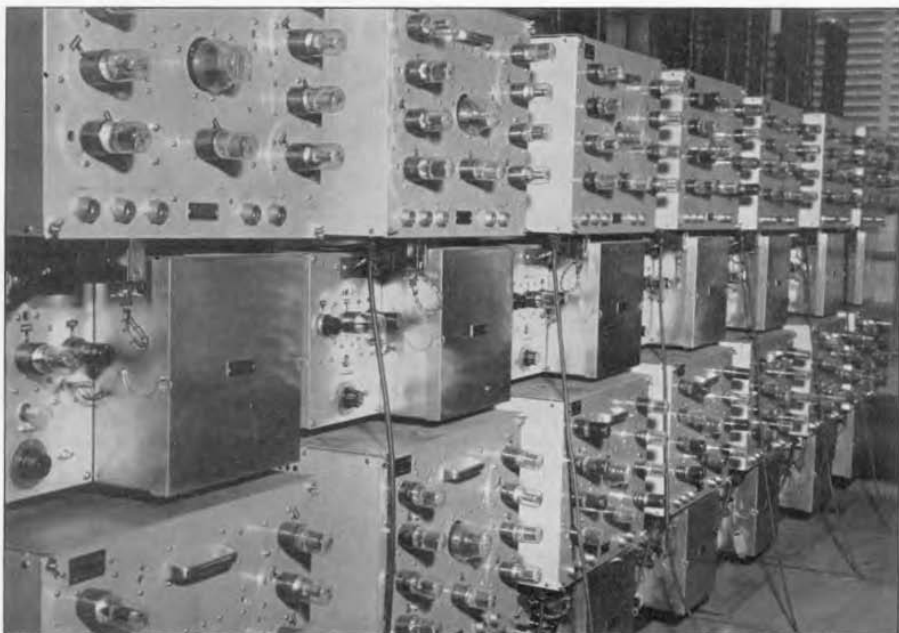
A group of Type 1100 Frequency Standards undergoing performance tests in our Standardizing Laboratory. Accuracy and stability must be well inside catalog specifications before the oscillators receive the Laboratory's O.K.
