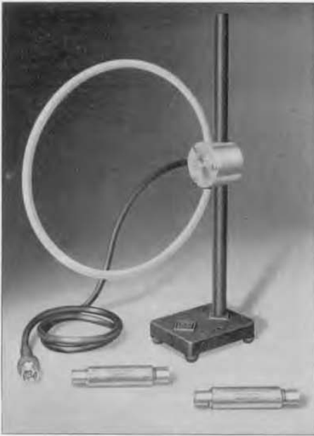
Figure 10. View of the Type 1000-P10 Test Loop, the Type 1000-P3 Voltage Divider, and the Type 1000-P4 Standard Dummy Antenna.
