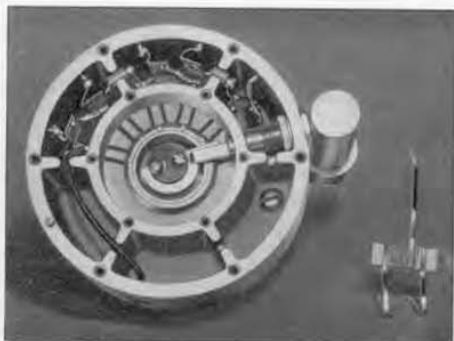
Figure 8. View of the casting that houses the MULTIPLIER network. One of the mica cards, with a series and a shunt element of the ladder network wound on it, is shown at the right.
