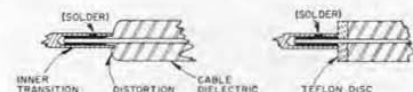
(Left) Figure 2. Typical soldering-heat distortion of cable dielectric. (Right) Figure 3. Teflon disk eliminates distortion.
