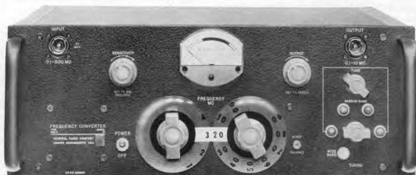
Figure 1. Panel view of the Type 1133-A Frequency Converter.
