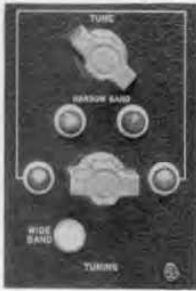
Figure 3. Tuning controls. Signal lights indicate proper setting.
