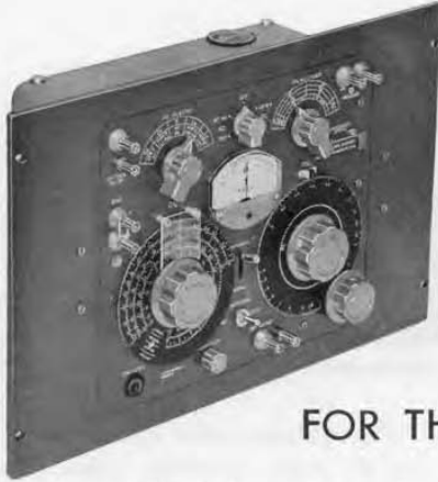
Figure 1. The new relay-rack model of the Type 1650-A Impedance Bridge.
