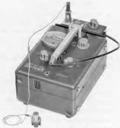
Figure 3. View of the Type 1560-P11S2 Vibration Pickup System with the Type 1551-C Sound-Level Meter.
