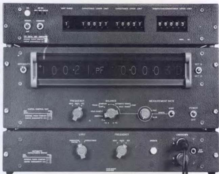
Figure 1. GR 1781 Digital Limit Comparator shown with automatic bridge.
