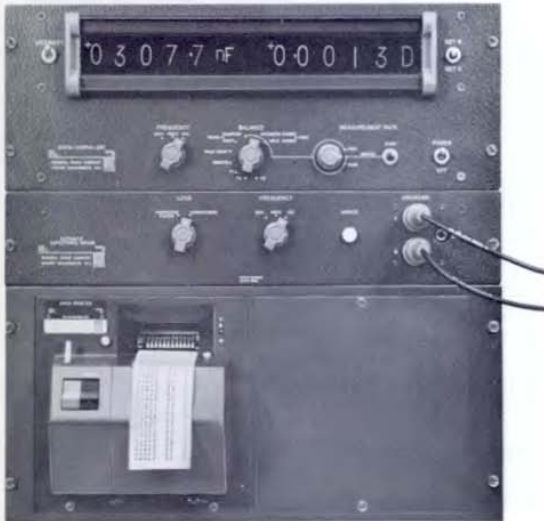
Figure 2. Automatic capacitance bridge and data printer.
