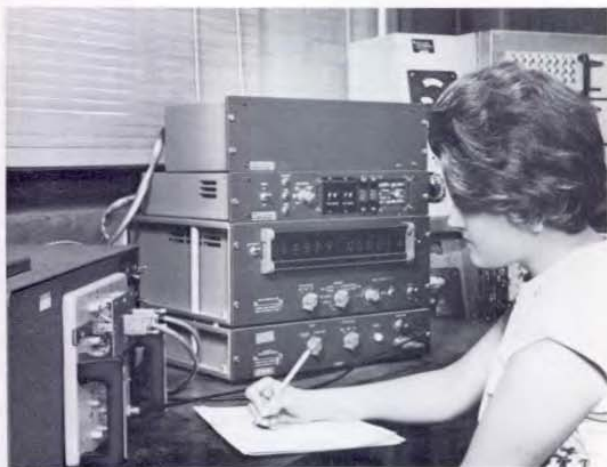
Figure 6. Bridge-scanner system used in environmental tests on dipped-mica capacitors.
