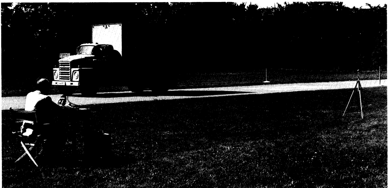
Figure 2-12. Remote location of microphone on tripod is demonstrated by this motor-vehicle noise measurement setup.
