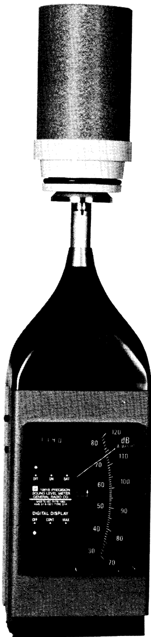
Figure 2-2. Calibration, with the 1567 Sound-Level Calibrator.
