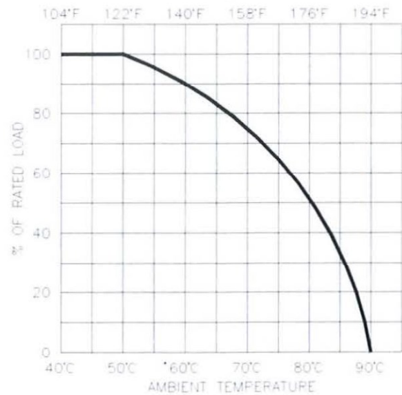
Figure 2 Ambient Temperature Derating Curve
