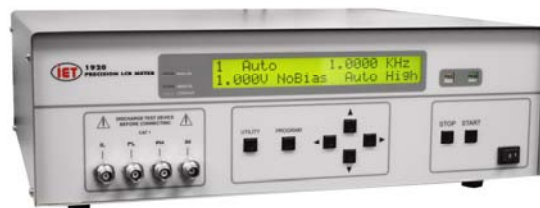
Figure 4: IET Labs 1900 Series Precision LCR Meter
