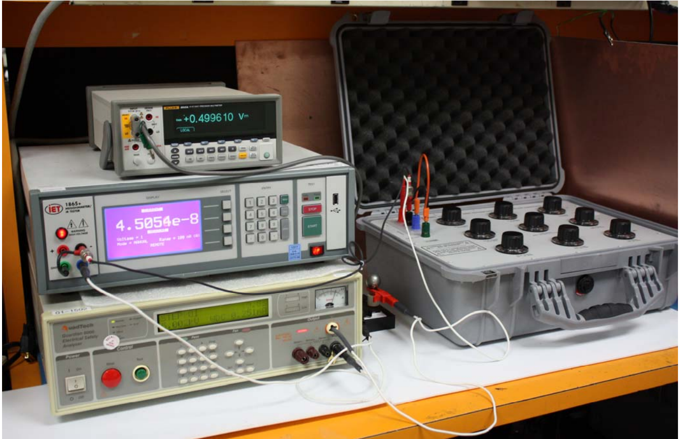
Figure 3: MegBridge in measuring resistance on a HRRS High Voltage Decade Resistor
