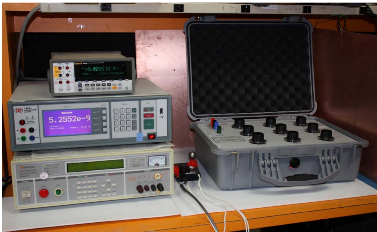
Figure 1: Instruments used for system along with IET Labs HRRS High Voltage Decade Resistor
